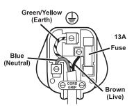
Ensure that the outer sheath of the cable is firmly held by the clamp
